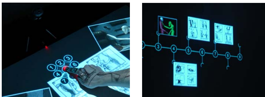
Figure 6: A virtual number block is projected on the surface after a double-click onto data.
